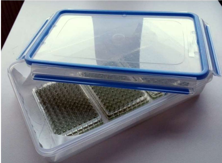
Fig. 2 Exemplary storage box with paper towel, holding 3 Multiwell plates
