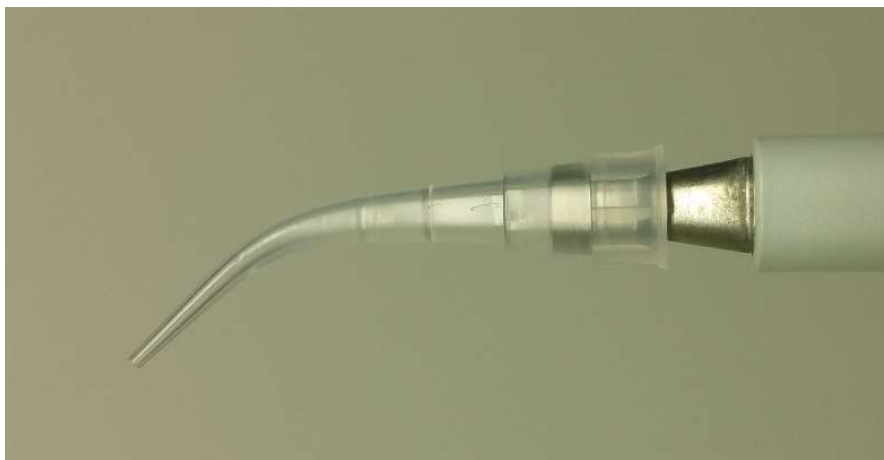
Fig. 1 Kinked 10 µl pipette. The tip was softened using a crème-brule burner and a forceps.
